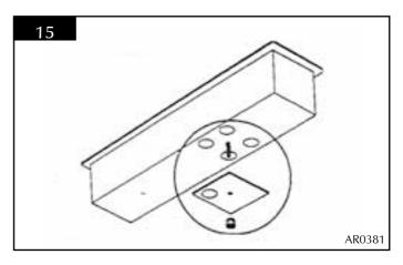
10.3 Remove the plate and replace with the correct size, ensure that the hole(s) in the plate align correctly with the holes in the underside of the airbox and replace the Nyloc nut.
